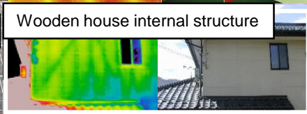
Defective spots of heat insulation material
